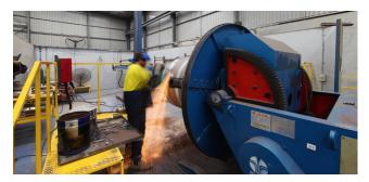
2. Back Grinding (Section Replacement)
